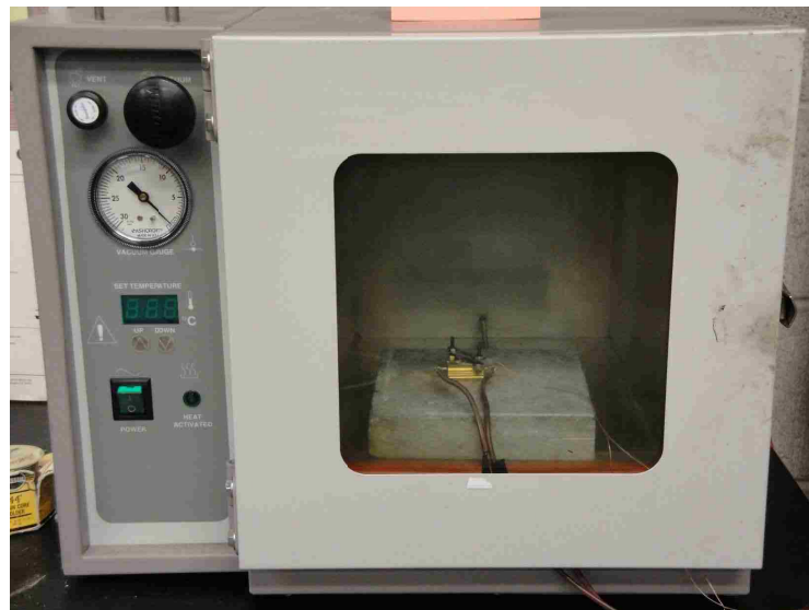
Figure 16 Ambient Pressure Setup for Transport Properties
