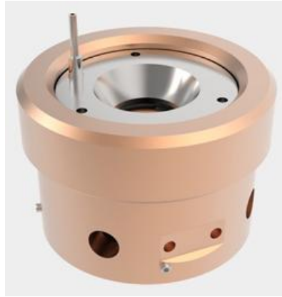
Figure 26. Almax-Easylab CuBe non-magnetic Pressure cell. Has a build-in gas membrane drive.
