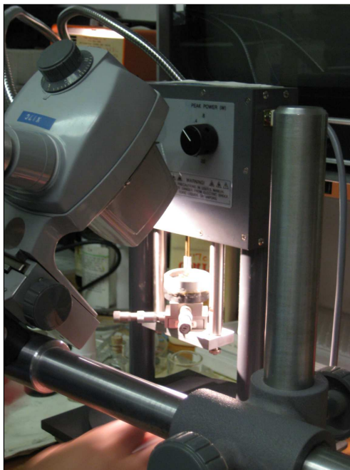
Figure 8: EDM, showing alignment stereo microscope
