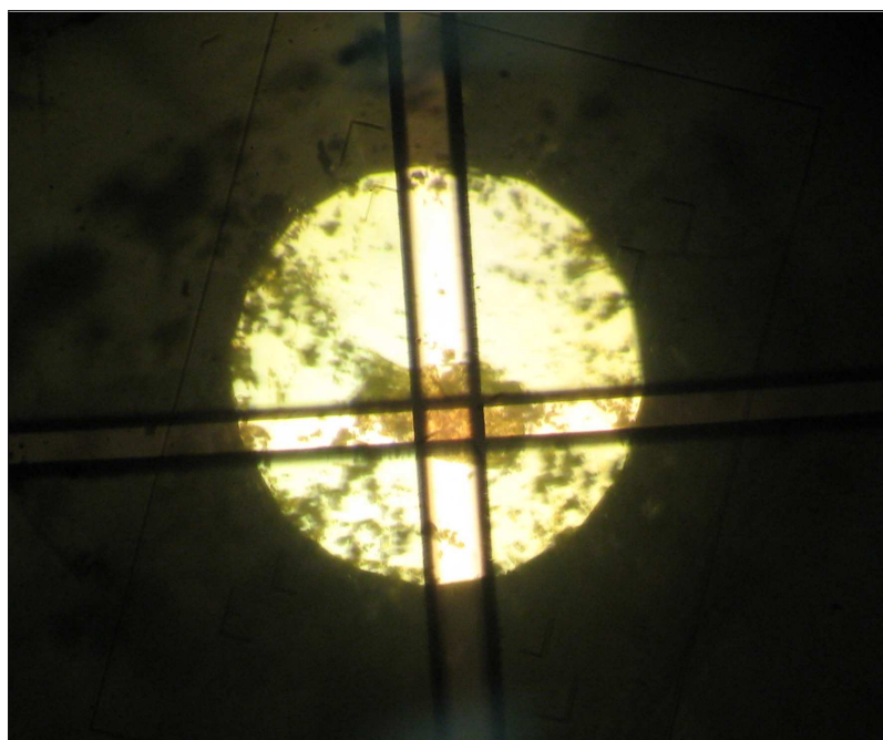
Figure 10: TATB powder on diamond culet, through microscope
