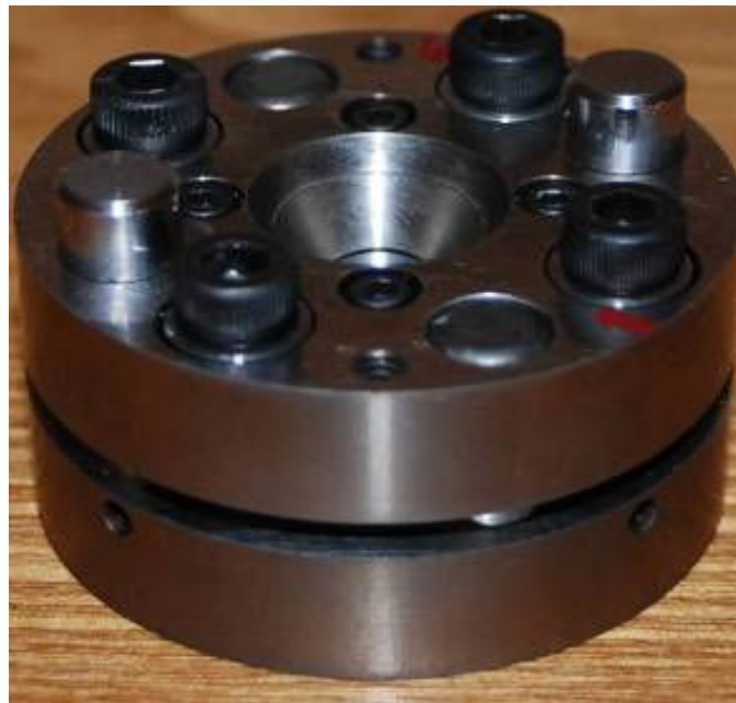
Figure 6. Top picture - Front left: Four pin DAC, bottom part with the Re gasket covering the bottom culet. Front right: Four pin DAC, top part with top culet. Rear left and right: Load screws with Belleville washers. Bottom picture – Assembled DAC.
