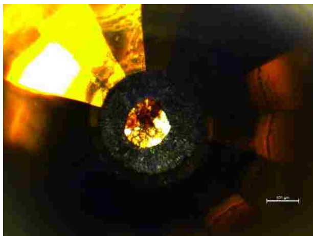
Figure 5.3: Image of irradiated mixture of CsF and \text{KBF}_4 pressurized to 70 GPa.
