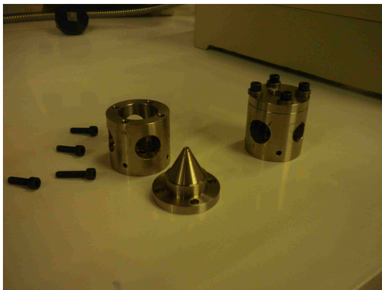
FIGURE 3.3: A picture of two jigs, one open and one closed. This device presses the bottom face of the diamond against the diamond seat while allowing the seat to be translated until the seat axis and diamond axis coincide. The openings on the perimeter allow one to apply glue where the diamond meets the seat.
