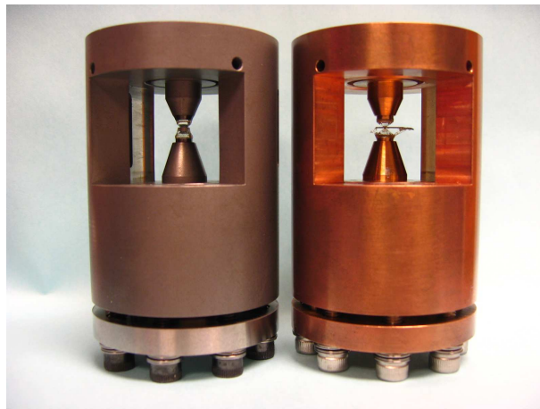
Figure 19 Paderborn-panoramic style diamond anvil cell.
