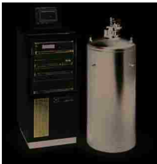
Figure 5 A Quantum Design Physical Property Measurement System, with an interior view of the dewar.
