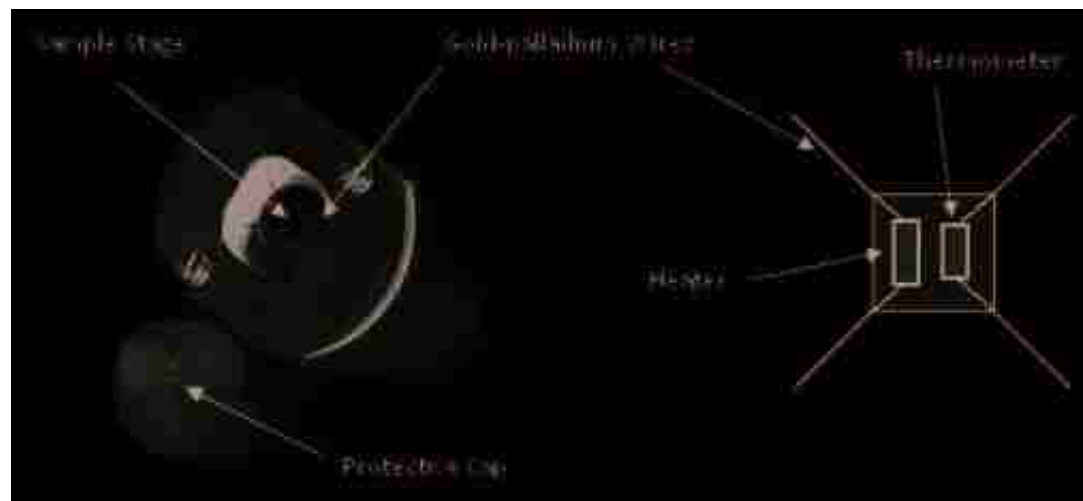
Figure 7 A Helium 3 Heat Capacity Puck. The left image shows the placement of the heater and the thermometer on the underside of the stage on which the sample is placed.
