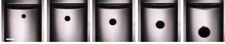
Figure 5.2. Static Stokes experiment showing the depths of submersion of Silicon Nitride Ceramic balls of diameters 2.4mm, 3.2mm, 4mm, 4.8mm and 6.35mm respectively in a 3.1% PAM hydrogel. The white scale bar represents 5mm.
