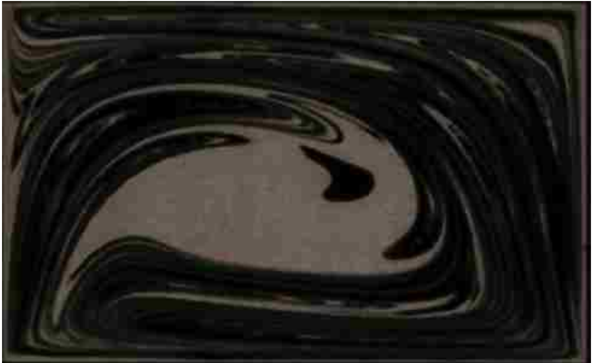
Figure 5.2: Chaotic mixing in a cavity flow (Ottino, 1990).
