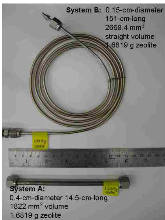
Figure 3.4: Systems A and B with different adsorber packed bed geometries and volumes but contained same amount of zeolite with the same particle sizes.
