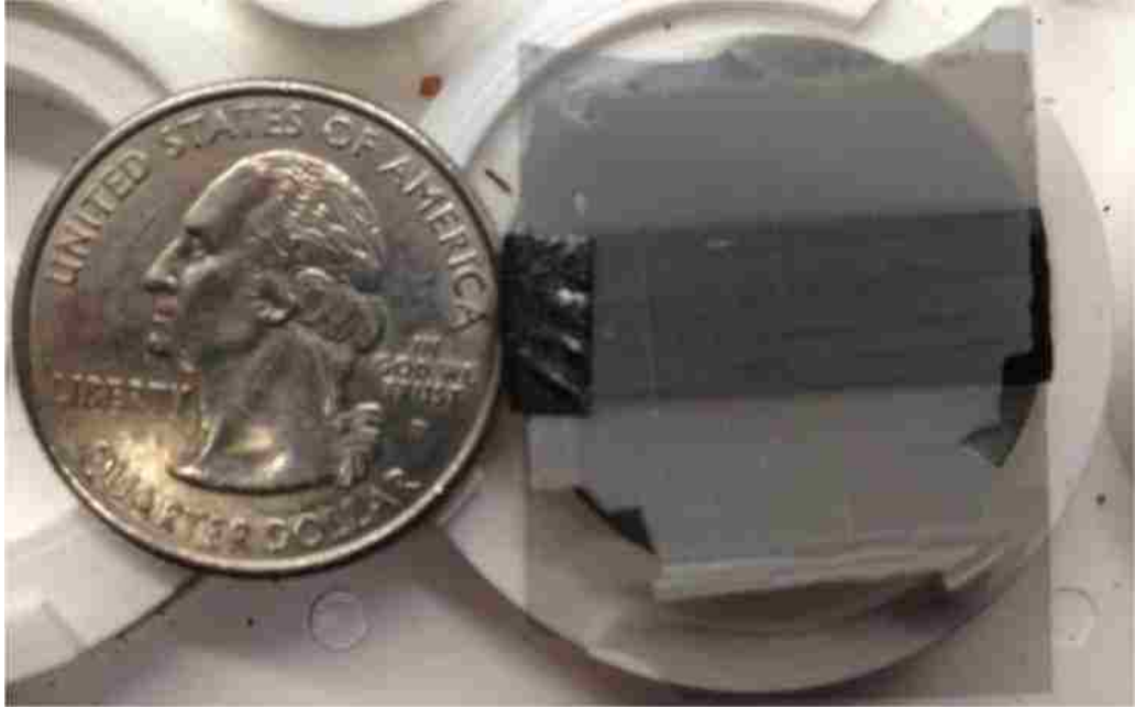
Figure 7.8: Photo showing a six-layer membrane, synthesized through three depositions at \frac{1}{2} v_{\text{mono}} , prepared for SEM analysis. Membranes are mechanically strong enough to be easily handled.
