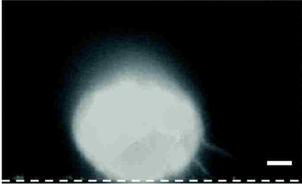
Figure 6.8: A confocal Z-stack image showing tethers from a Rhodamine B stained Jurkat cell to an antibody functionalized smooth glass substrate (scale bar = 2 \mu\text{m} ). After cell capture from continuous flow on an antibody-treated smooth glass slide, the flow was stopped and confocal images were acquired. The fluid flowed from the right to the left for cell capture, and the substrate is located at the bottom of the image as indicated by the dashed line. The fuzziness of the membrane away from the substrate is a result of spontaneous membrane fluctuation.
