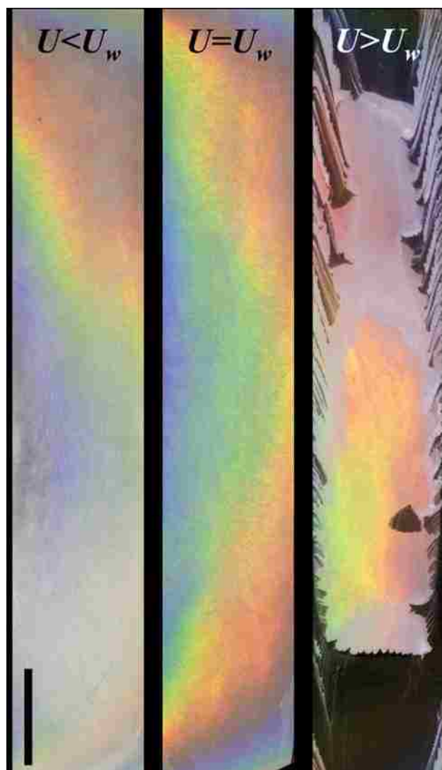
Figure 6.2 light scattering from different sample morphologies obtained with increasing substrate velocity, from left to right multilayer, monolayer and discontinuous. Scale bar corresponds to 5cm.
