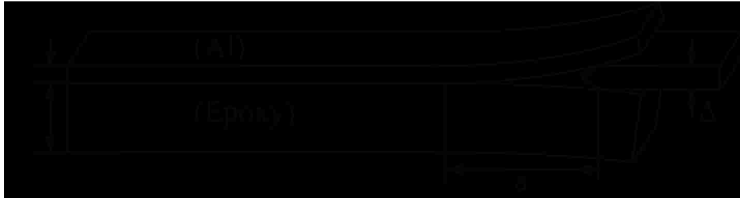
Figure 1.11: Schematic of the ADCB sample. E_1 , E_2 , h_1 , h_2 , a and \Delta correspond to the aluminum elastic modulus, epoxy elastic modulus, aluminum thickness, epoxy thickness, crack length and wedge height.
