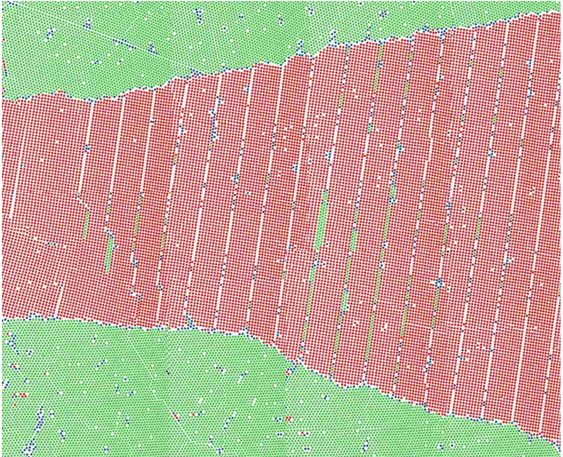
Figure 4.15: Reconstructed panorama image of defect pattern which shows the defects running along the minor dimension of the crystal
