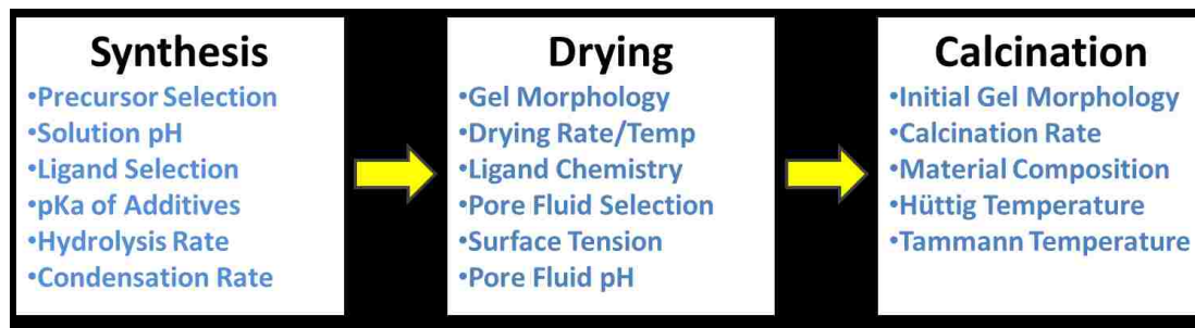
Figure 1-7. Key processing parameters during synthesis and preparation of a catalytic supported oxide.
