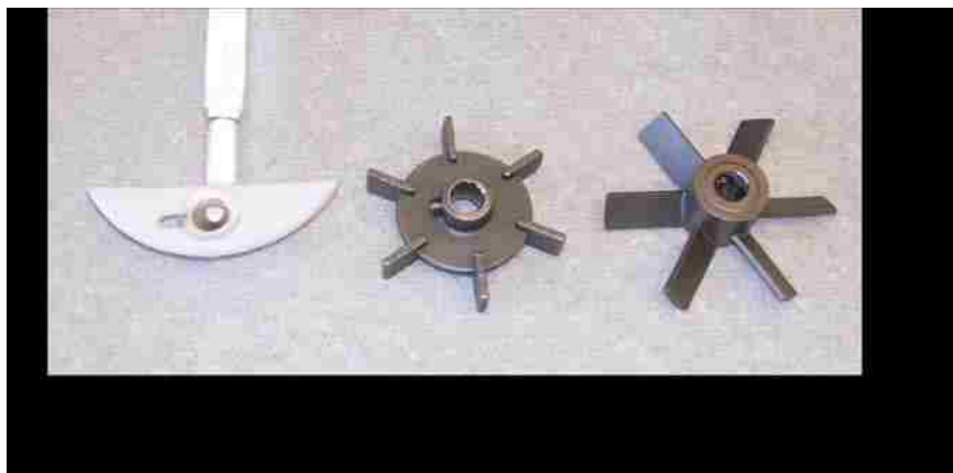
Figure 3.3: Three different impellers used in semi-batch adiabatic redox-initiated emulsion polymerizations.
