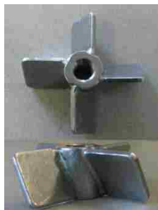
Figure 4.5: Pitched-blade impeller used in Mettler RCI reactor.
