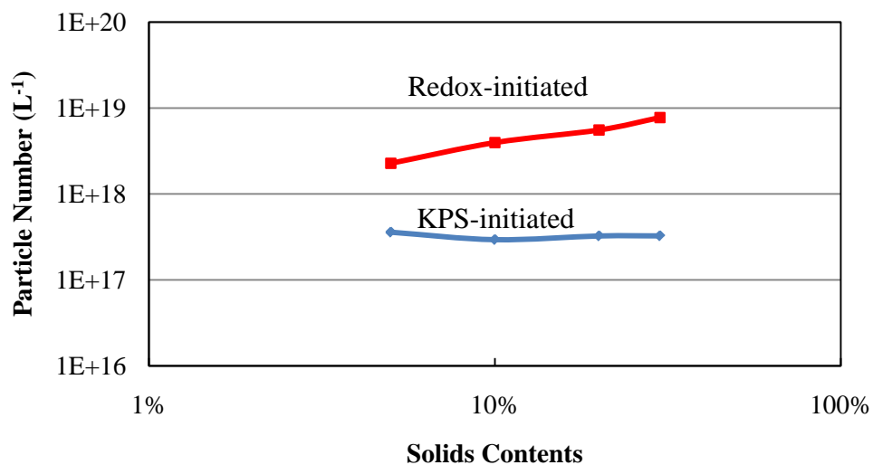
Figure 4.37: Log-Log plot of particle number versus solids contents for KPS-initiated and redox-initiated latexes.
