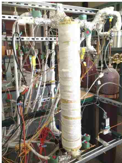
Figure 3-4 Picture of the pilot scale experimental setup for high temperature PSA test of CO 2 capture
