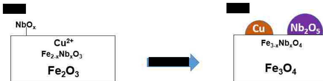
Figure 6.12. Schematic of the supported 3Cu/8NbFe catalyst (a) calcined and (b) during HT-WGS
