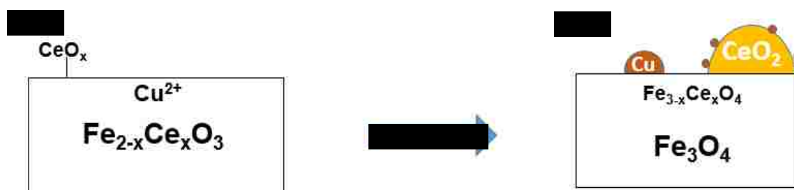
Figure 6.17. Schematic of the 3Cu/8CeFe catalyst (a) calcined and (b) during HT-WGSR
