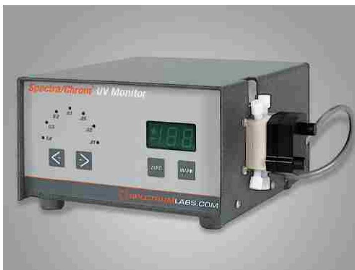
Figure 1.4: UV detector for in-line solute analysis (Copyright Spectrum, Inc.)
