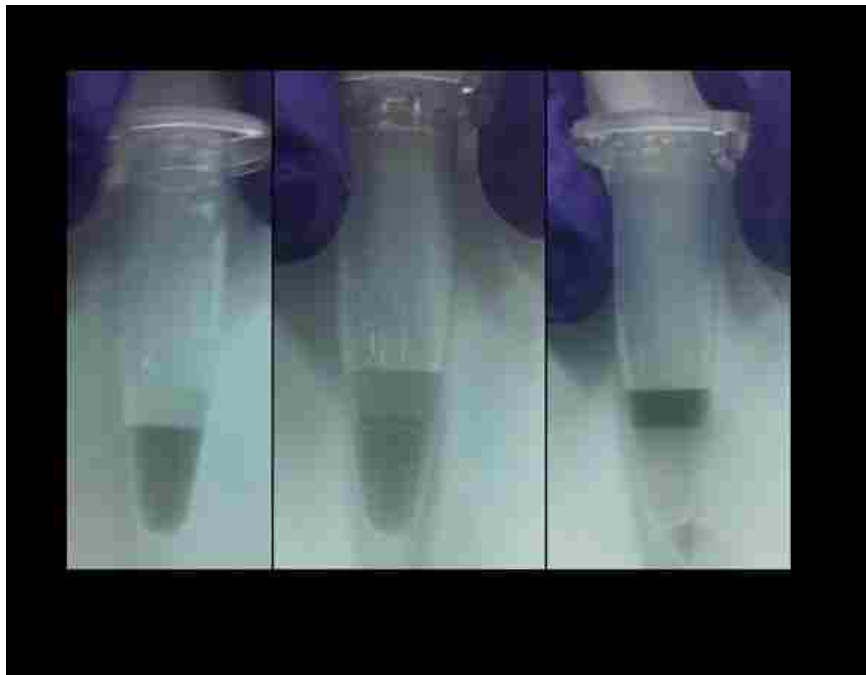
Figure 3.1 With the addition of PVP, the DNA-CNT hybrid moves from being mostly in the bottom phase to mostly in the top phase
