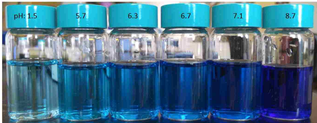
Figure 20: Photograph of a 100mM copper nitrate and 200mM lactic acid solution as pH increases. It should be noted that the solution remains clear throughout the transition from lactic acid bound cerium at low pH to ammonia bound cerium at high pH, with no solid cupric hydroxide formation in the intermediate pH range.
