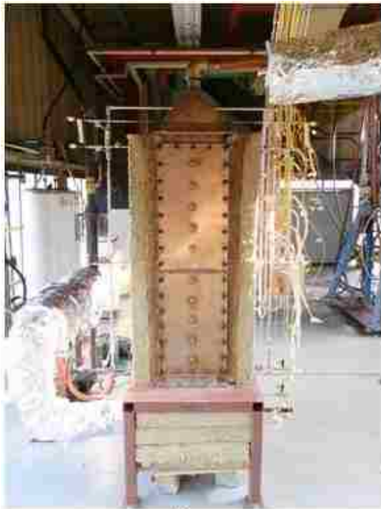
Figure 4-27. The test facility with EPCM based TES system for process demonstration. (a). schematic of the general test loop (without insulation); (b). a photo of the test section with insulation (the front insulation is removed); (c). a photo of the encapsulated \text{NaNO}_3 capsules in the test section.
