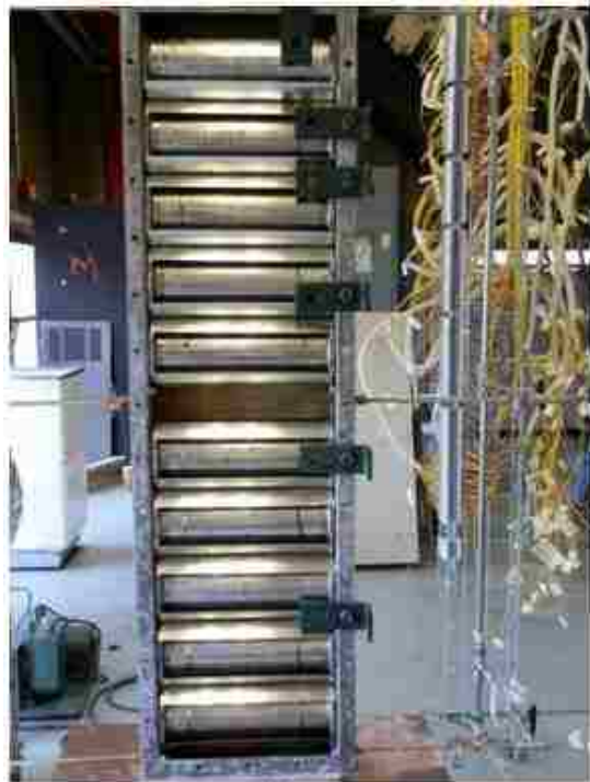
Figure 4-27. The test facility with EPCM based TES system for process demonstration. (a). schematic of the general test loop (without insulation); (b). a photo of the test section with insulation (the front insulation is removed); (c). a photo of the encapsulated \text{NaNO}_3 capsules in the test section.
