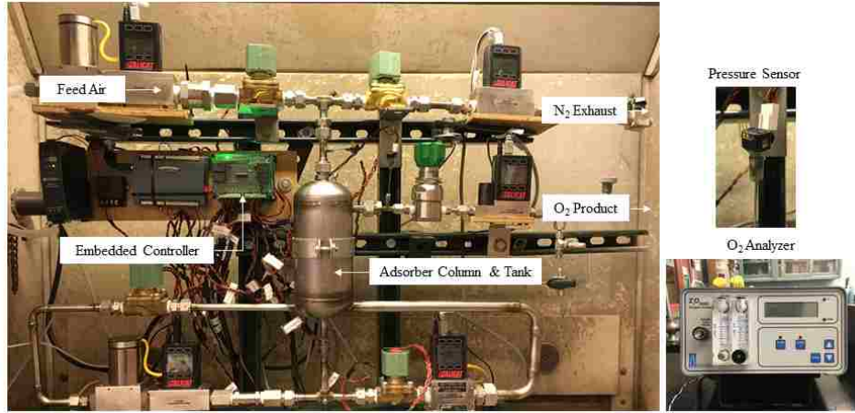
Figure 5.1: Lab-Scale MOC Device with Embedded Controller: The single-bed RPSA device uses a single adsorber column inserted concentrically into a product storage tank. Feed air is supplied from a compressed-air source, and high purity O_2 product exits the storage tank.
