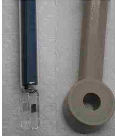
Figure 1.1: Resistance conductivity probe (left) and torroidal probe (right).
