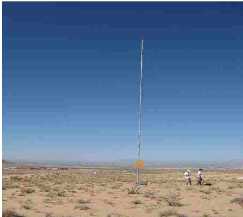
Figure 1.4 Towers to measure the wind data
