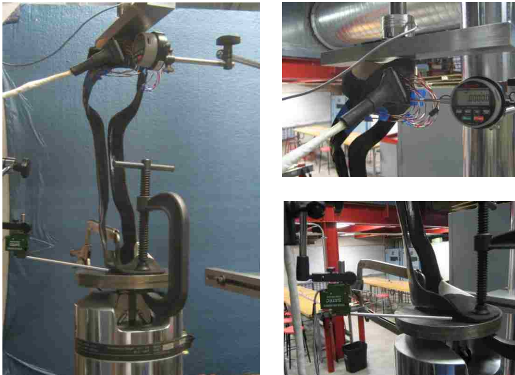
Figure 4.4: Actual test setup for vertical compression test
