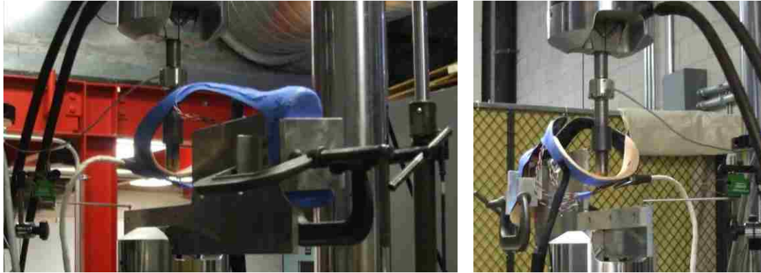
Figure 4.3: Actual test setup for horizontal cantilever flexure test
