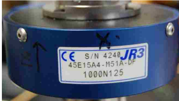
Figure 3.1: JR3 45E15 Transducer
