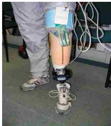
Figure 10.2: Experimental setup of transducer and F-socket.
