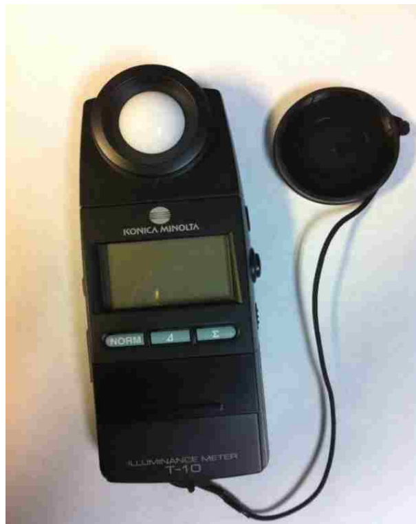
Figure 3.17 Konica Minolta illuminance meter T-10
