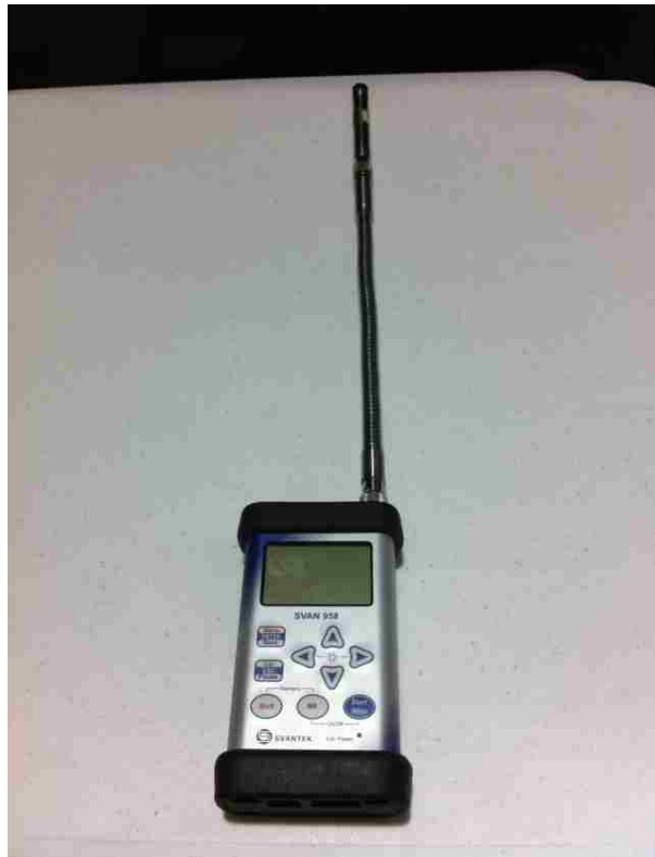
Figure 3.18 Svantek 958 four channel sound and vibration analyzer
