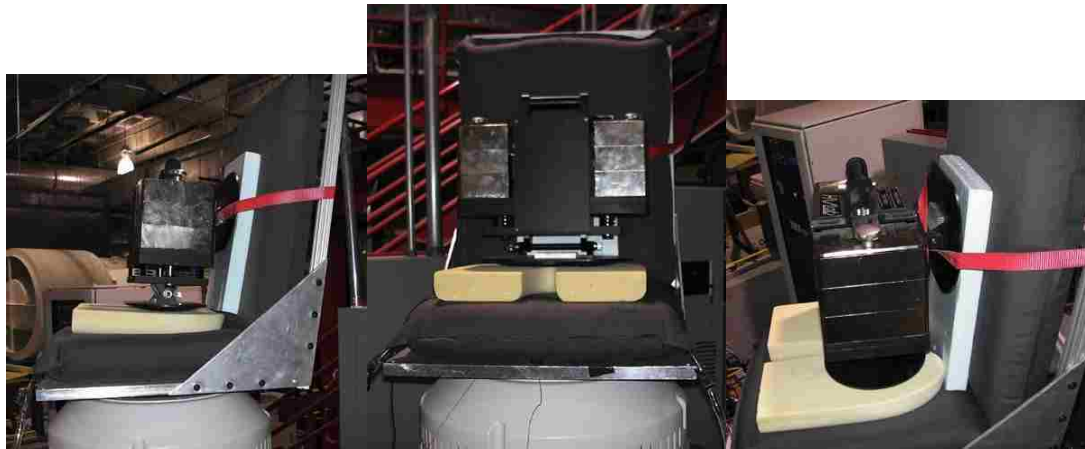
Figure 4.1 Experimental Setup for Seat Vibration Transmissibility
