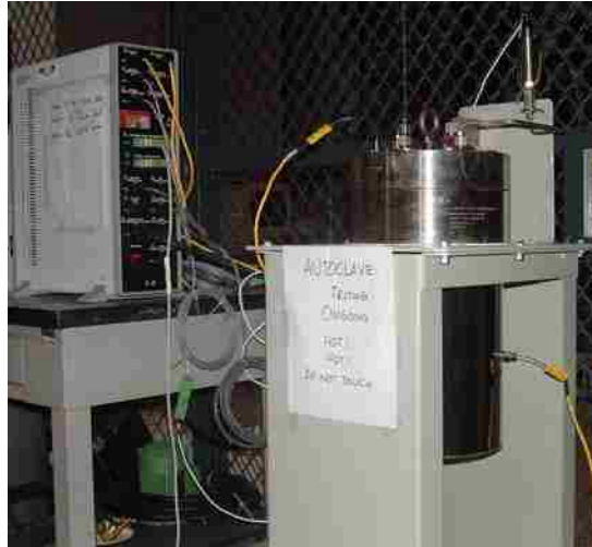
Figure 3-14 DCB Test Setup
