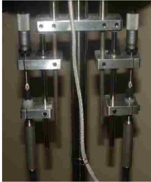
Figure 3-2 Extensometers used in Creep Testing
