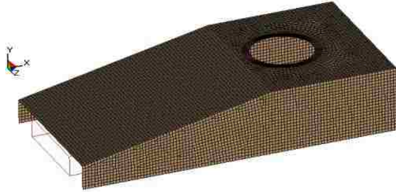
Figure 2.11: FE model of the vehicle with the internal space frame
