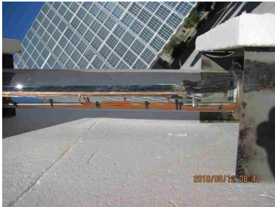
Fig. 12 Thermocouples attached to back of the cells
