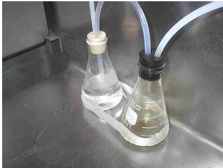
Figure 3.7 Condensate and particulate trap
