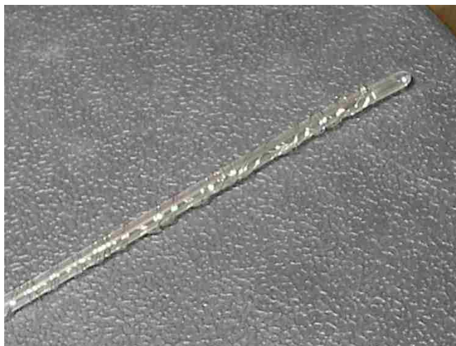
Figure 3.8 Nickel catalyst ready for insertion into system
