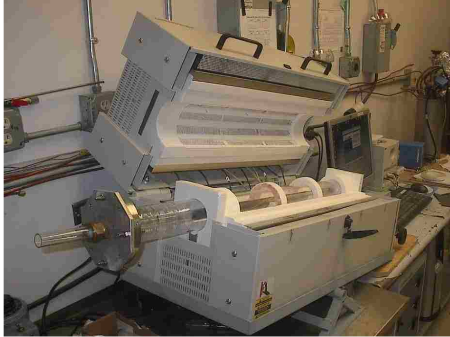
Figure 3.4 Containment tube with process tube (gen 2)
