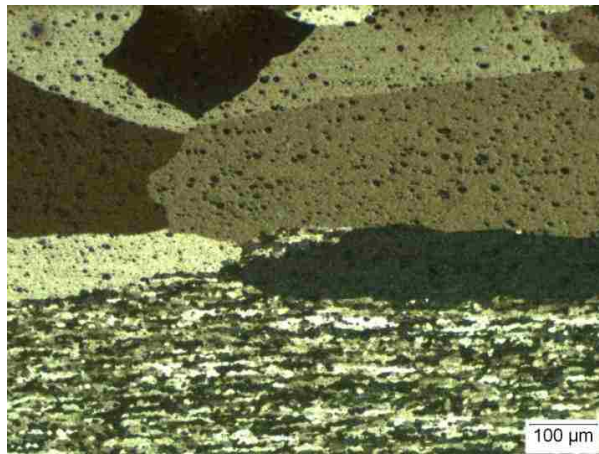
Figure 17. Light Optical Microscopy images for the thickest part of the extrudate extruded with the ram speed 2mm/sec (a) top (b) center (c) middle
