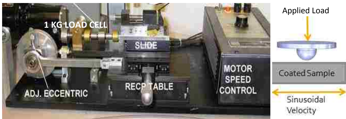
Figure 3-9: Friction Testing Apparatus [43]
