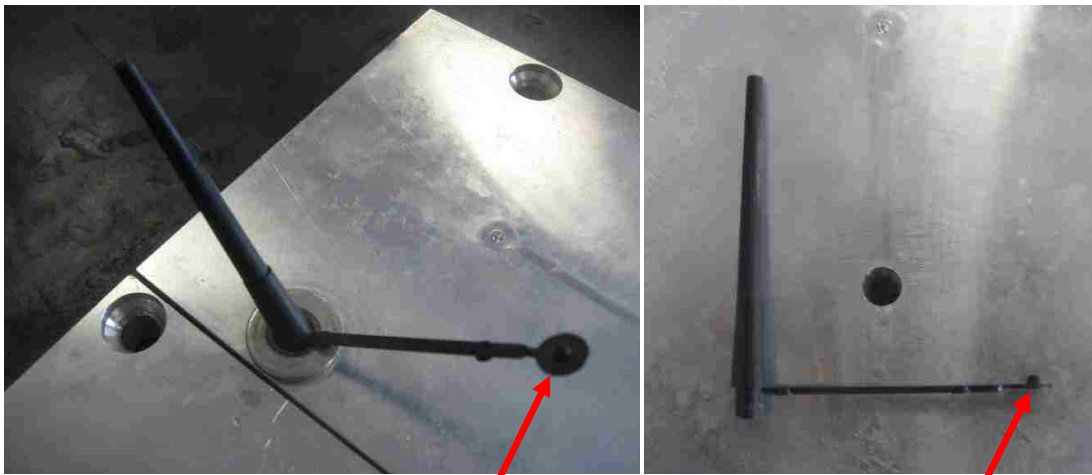
Figure 3-6: Image of Molded Part for Use in Pin-on-Plate Wear Testing and Friction Testing
