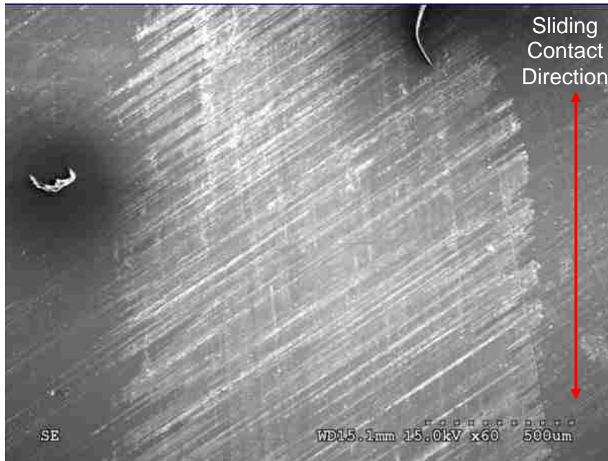
Figure 4-21: Wear Track on Electrodeposited Chrome Sample after 32,000 Repetitions of Sliding Contact against Copper Alloy Hemisphere with Applied Weight of 494.9 g
