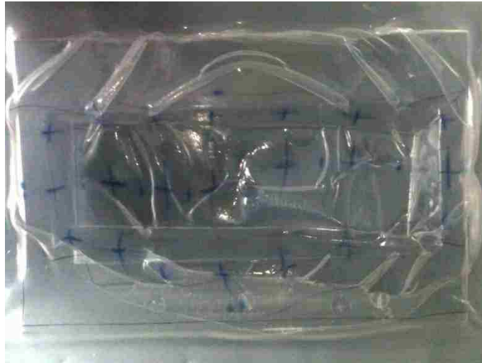
Figure 26 Forming failure on pure elastomer
