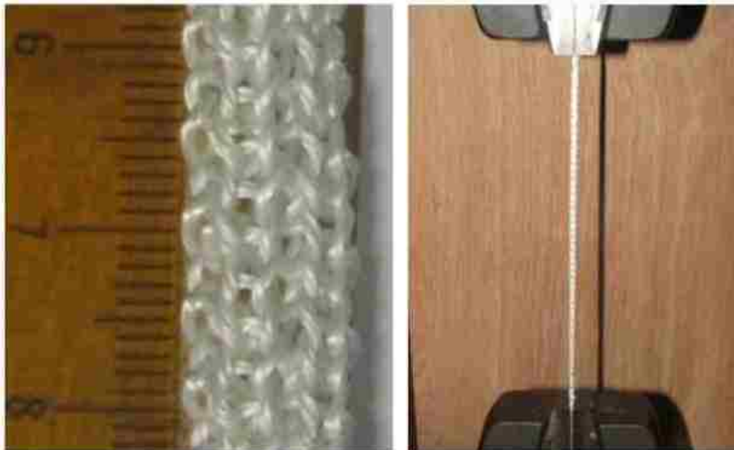
Figure 14 Uniaxial tensile tests on knitted fabric
