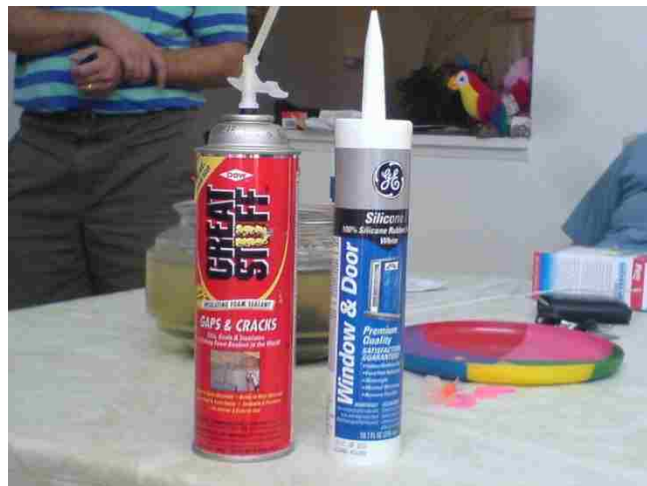
Figure 13. Insulating foam sealant used in duct sealing
