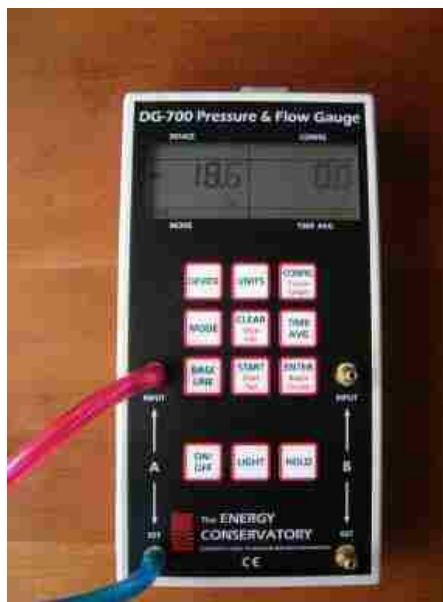
Figure 4. Pressure and flow gauge made by Energy Conservatory
