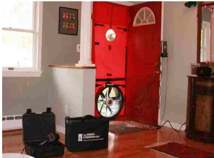
Figure 3. Typical blower door setup
