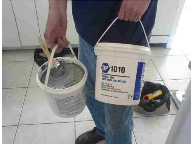
Figure 12. Smooth gray water based sealant used in duct sealing
