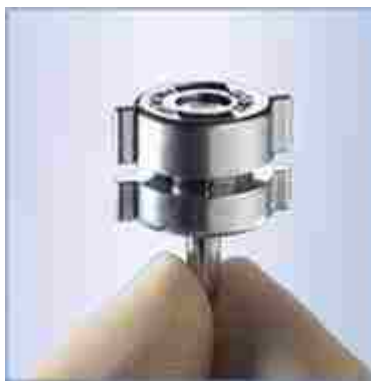
Figure 1: WetSEM Capsules used to view nanoparticles while suspended in fluids
