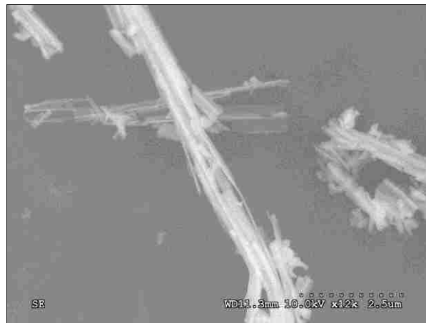
Figure 12: Sample 4A. Results for ten discs of 200 \mu\text{m} porosity with only fifteen 5mm grinding balls milled for five minutes at 300rpm using the planetary ball mill.
