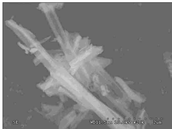
Figure 10: Sample 3A. Results for ten discs of 200nm porosity with thirty 5mm grinding balls milled for five minutes at 300rpm using the planetary ball mill.
