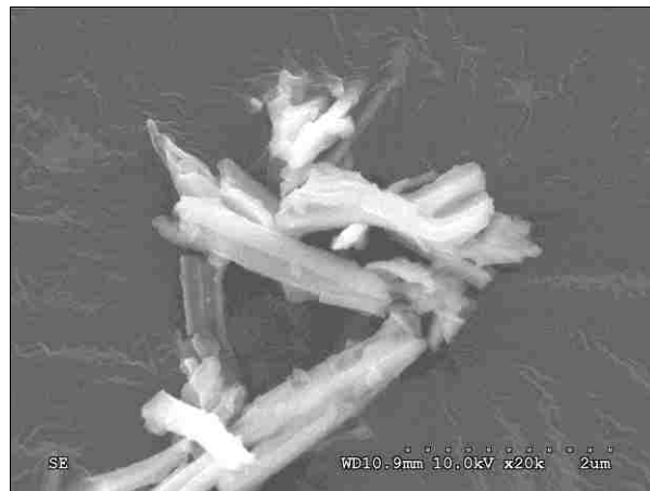
Figure 14: Sample 5A. Results for ten discs of 200 \mu m porosity with fifteen 5mm grinding balls milled at 300rpm for eight minutes using the planetary ball mill.
