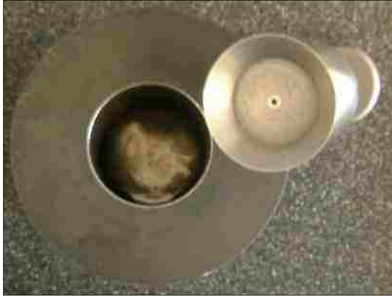
Figure 2: Couette Geometry used in the Ares Rheometer
