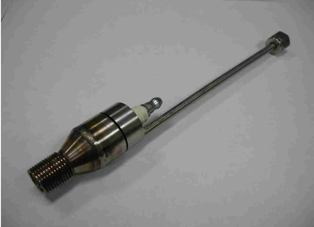
Figure 18. Second design spark plug/injector test assembly.
