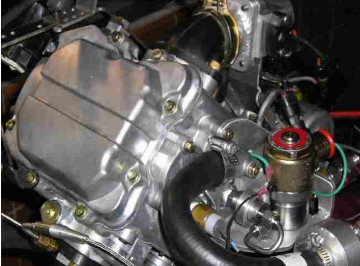
Figure 1. Polaris engine with direct injection hydrogen fueling. Figure courtesy of R. Fifield [6].
