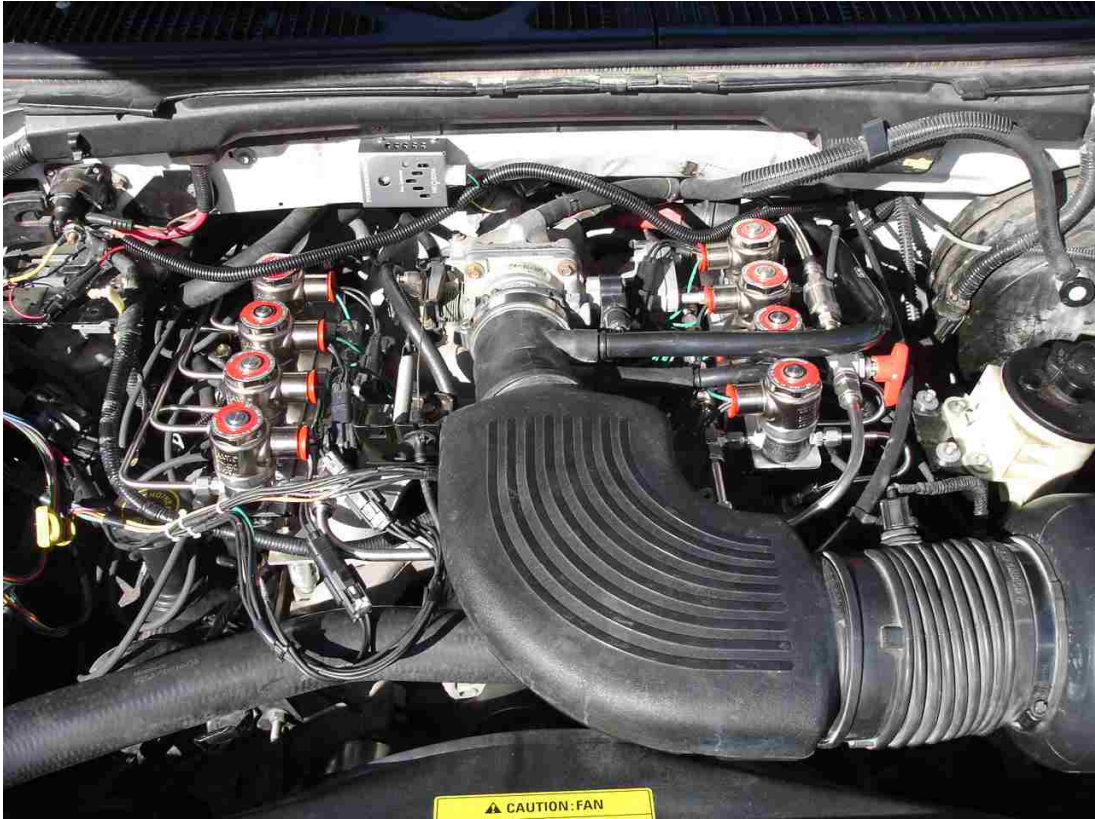
Figure 26. Completed installation of hydrogen direct injection system on Ford 5.4L engine.
