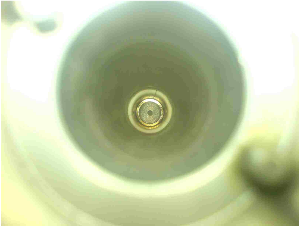
Figure 9. Visible cracking of lower electrode ceramic insulator.
