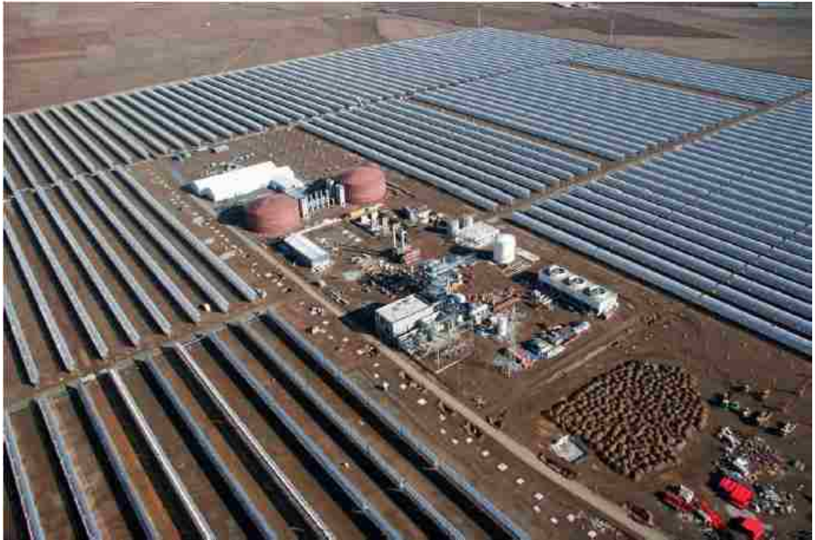
Figure 3: Thermal storage tanks at Andasol 1 [4]
