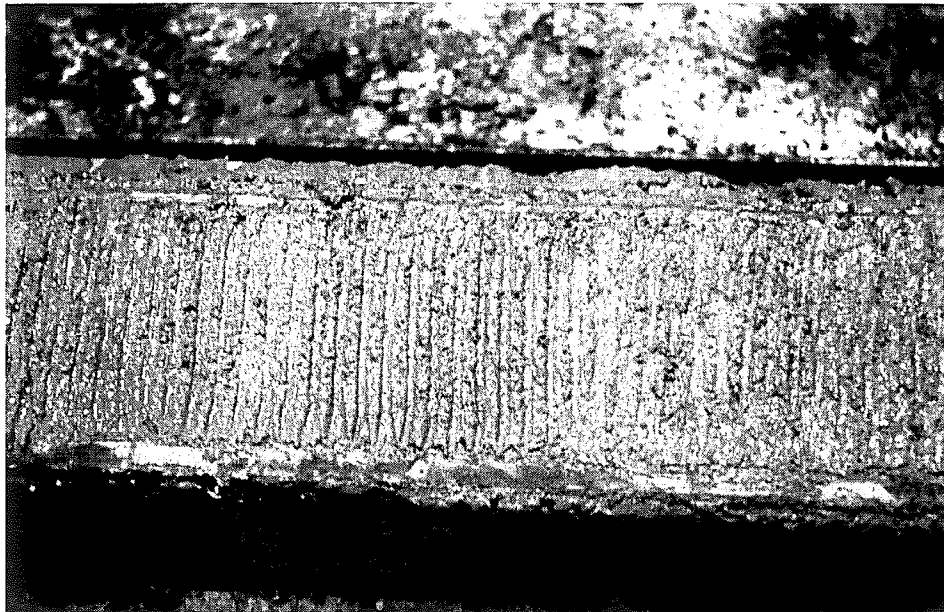
Figure 7-13: Rake Surface Finish
