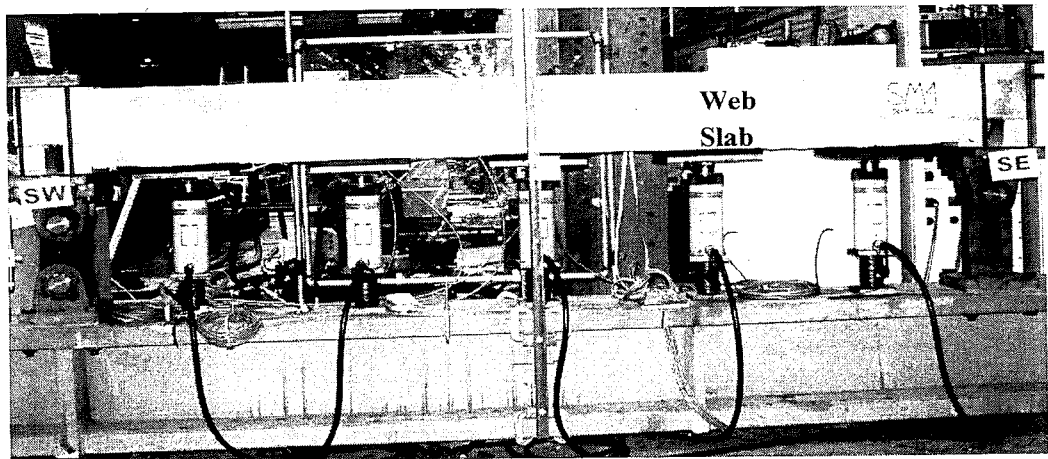
Figure 5-7: Five Point Load Configuration
