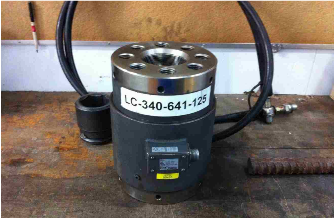
Figure 3-40 Load cell attached to the actuator
