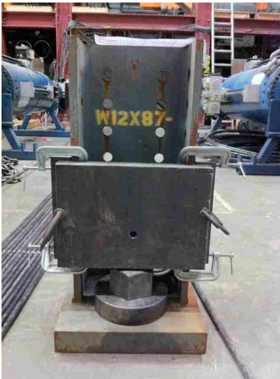
Figure 3-25 Setup for seating post-tensioning anchors
