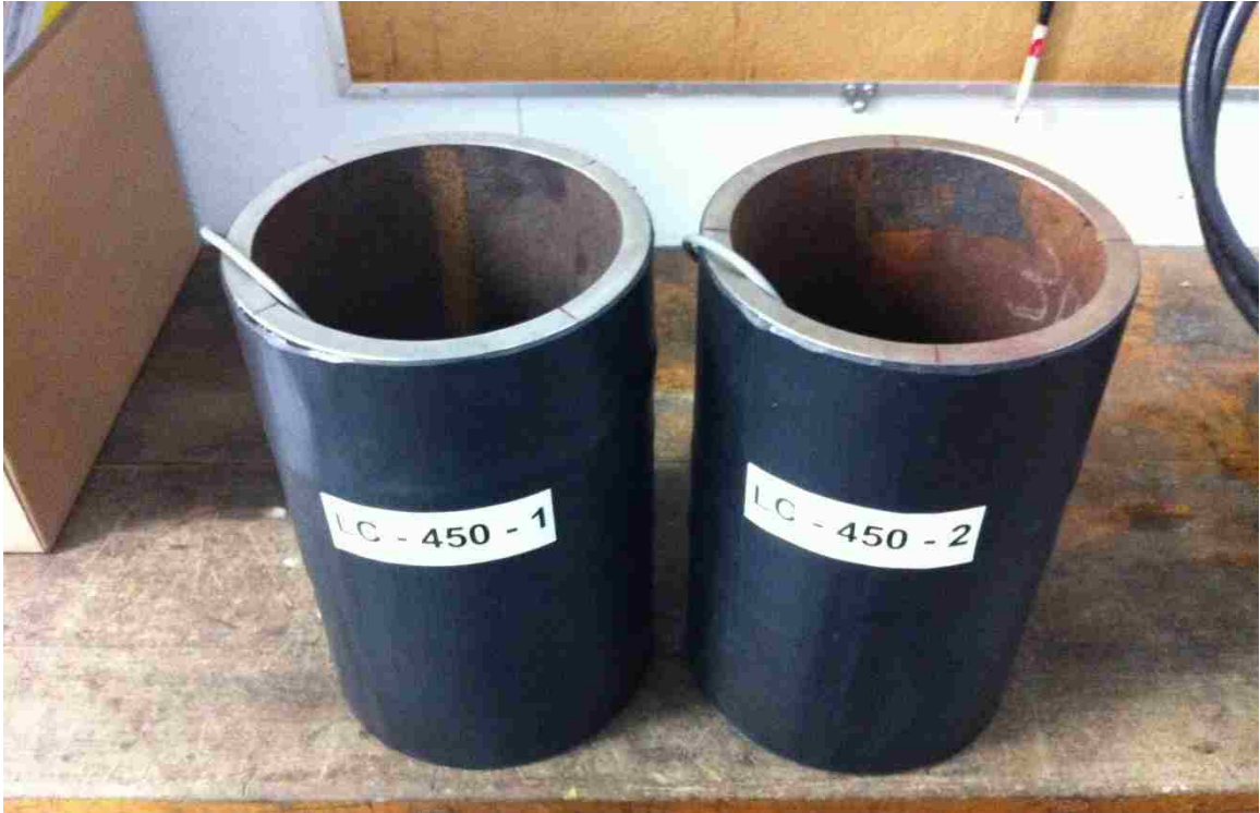
Figure 3-39 Load cells placed between the top anchor head encasement and the top of the wall
