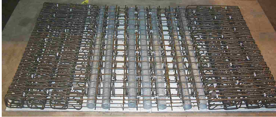
Figure 2-2 - Rebar Cage from Hoop-Confined Panel (Perez et al. 2004)
