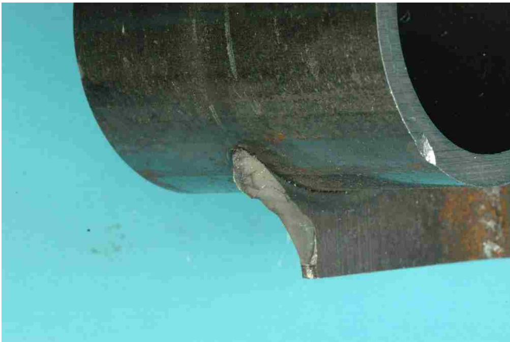
Figure 79. S9-T2 west crack plane, bottom half
