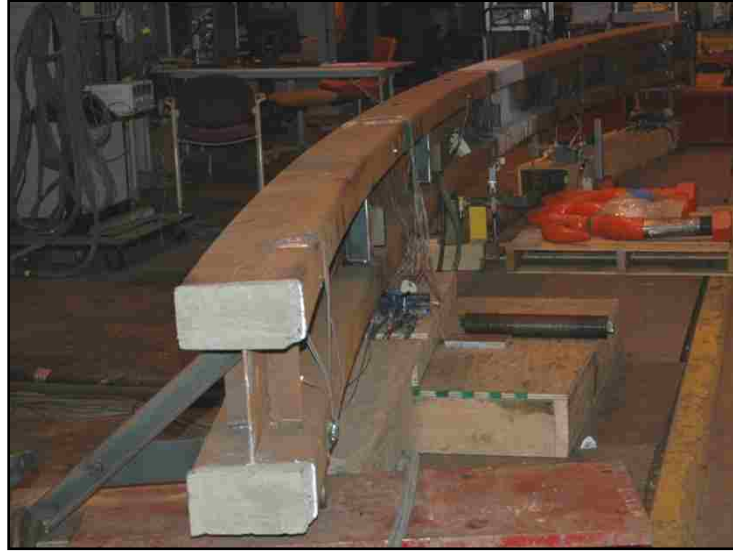
Figure 2.7: Curved TFG with hollow steel tube flanges and concrete infilled ends (Putnam, 2010)
