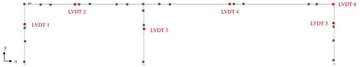
Figure 4.23. Simplified SAP2000 simulation with 29 nodes and 28 finite elements for static testing
