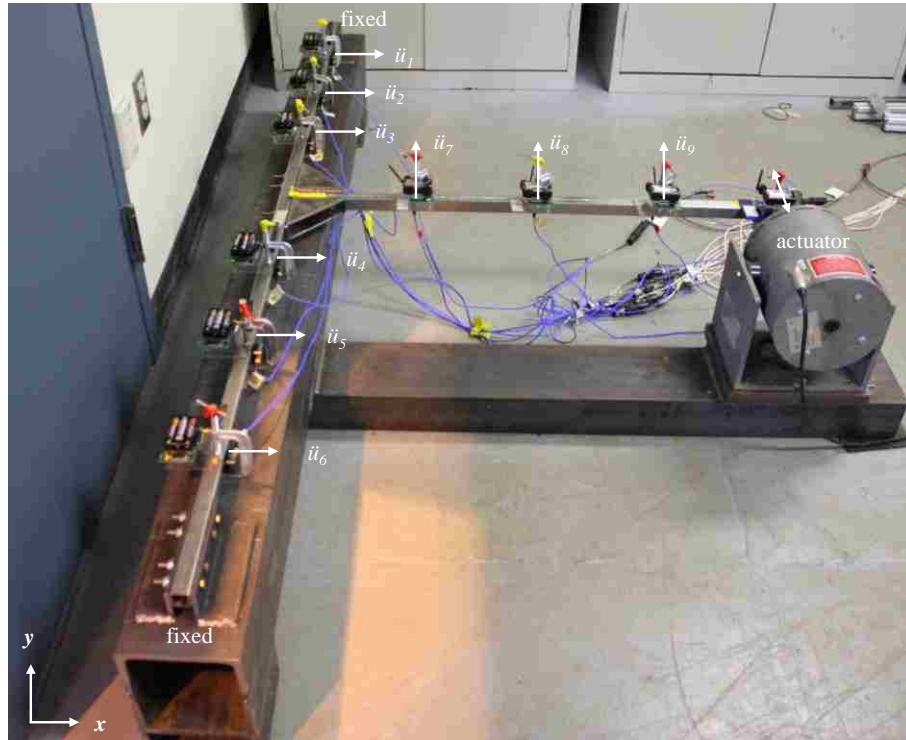
Figure 3.5. Experimental test bed for beam-column prototype instrumented with wired and wireless accelerometers
