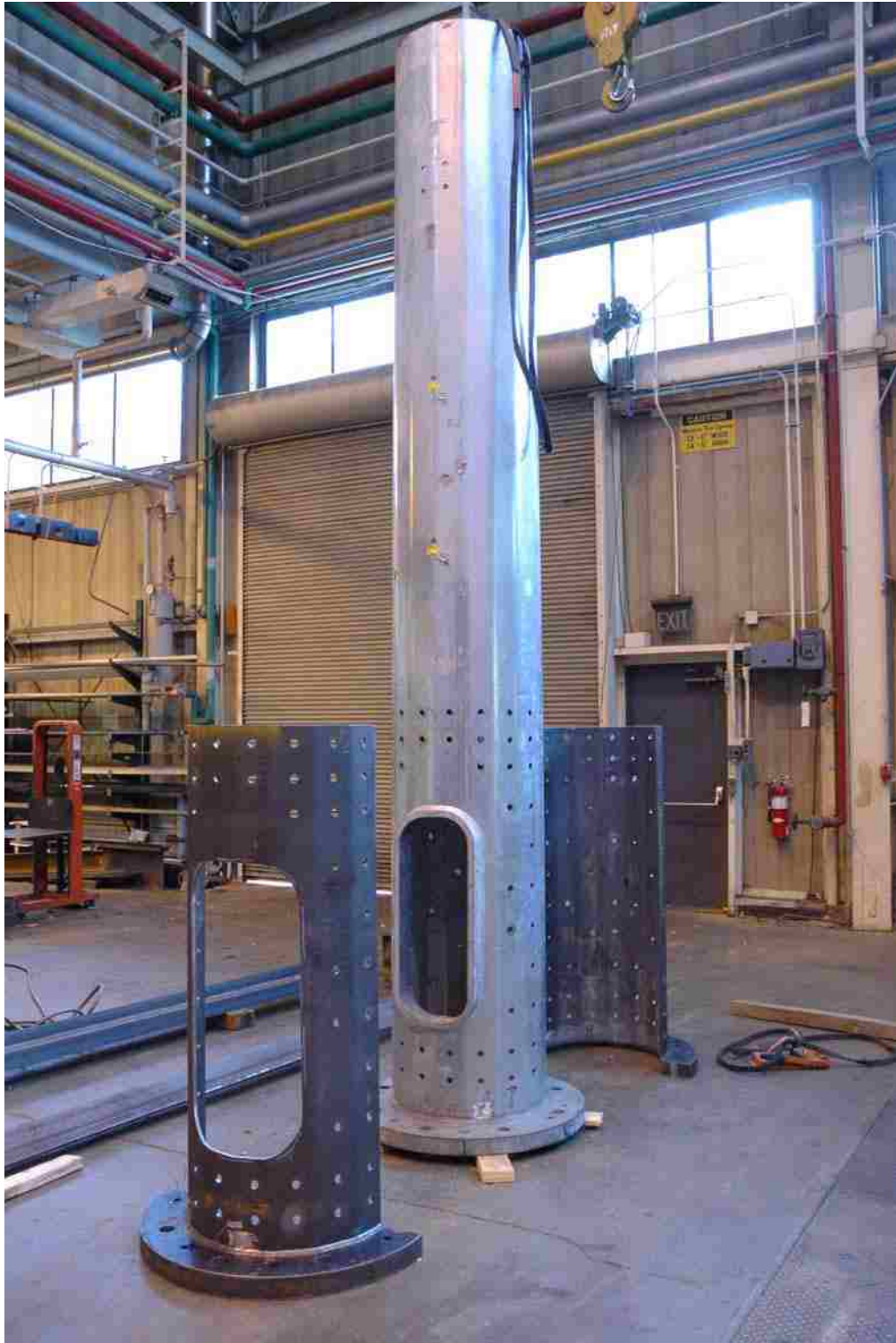
Figure 137. Retrofit jacket ready for connection to Specimen XI-9
