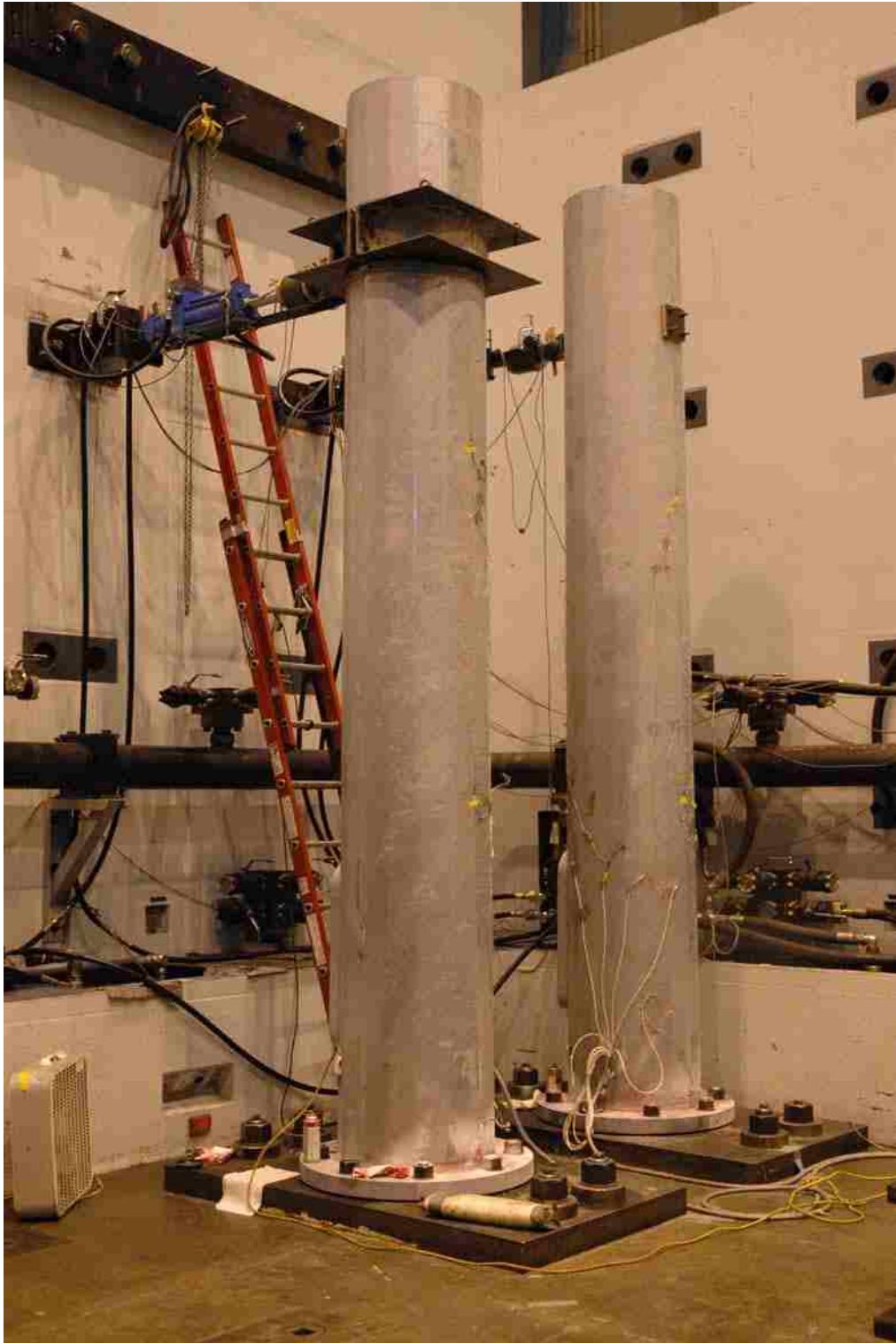
Figure 18. Fatigue testing setup at ATLSS
