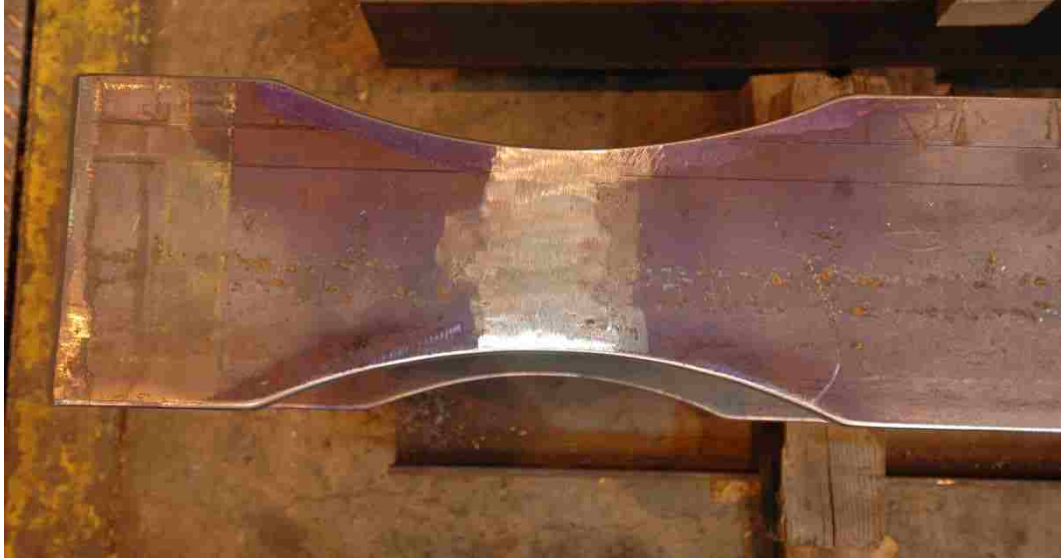
Figure 4.8 – Top view of 2 nd Floor Beam RBS cut
