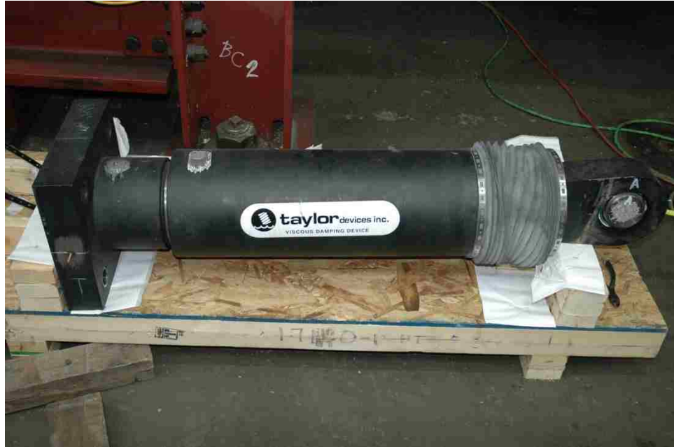
Figure 2.3 Viscous Damper Manufactured by Taylor Devices (Dong 2013)
