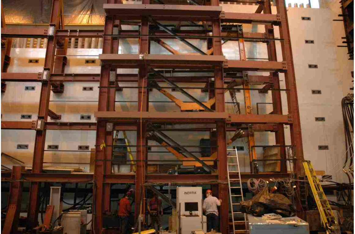
Figure 4.7- DBF in bracing frame
