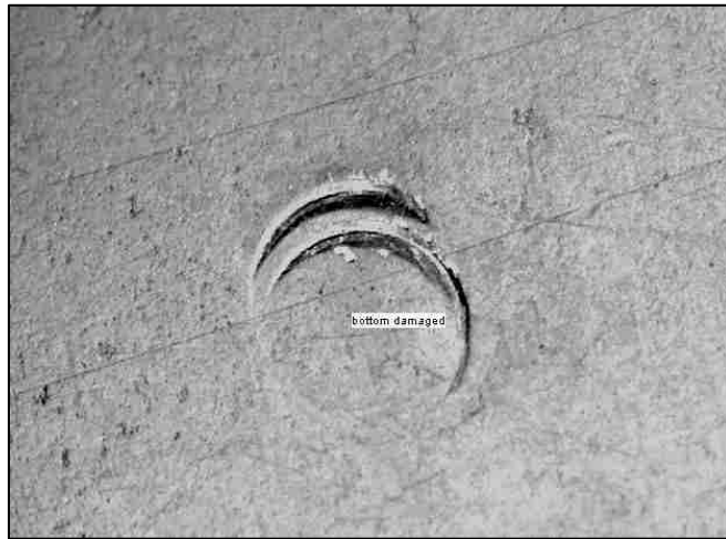
Figure 5.1: Damage on the back of a sensor that would impair it from working correctly
